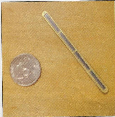
A photoconductive switch developed by BAE Systems—out of focus to avoid revealing details—uses laser-generated photons to switch electronic flow in an HPM weapon at the highest possible speed, enabling large power increases.
